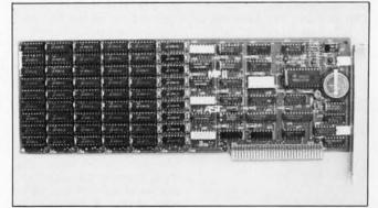
AST Research calls its MPII a "no frills" expansion card for the IBM PC XT. The MPII comes with 64K bytes of dynamic RAM, utility software, and a clock/calendar. Its memory capacity is upgradable to 348K bytes in 64K-byte increments. The price for the MPII ranges
