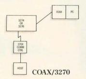
For instance, one solution is our Coax/3270. This single-slot expansion board lets you connect your IBM PC directly into virtually any IBM 3270 environment. And with our 3278/79 emulation software, it's easy to share information between your mainframe and IBM PC.
