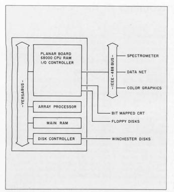
Figure 1: The architecture of the S9000 computer system used in the MIT NMR project. The 68000 CPU and SKY MNK-V array processor share access to memory over the VERSAbus. You can use as much as 2 megabytes of memory in imaging applications.
