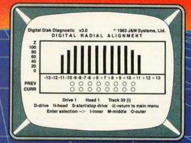
Use the DDA Radial Alignment Test to check the head alignment of your drives. No need for an oscilloscope or other expensive test equipment!
