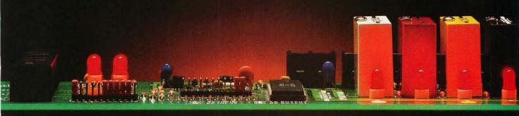
Opto 22, an IBM-PC Value Added Dealer, combines OPTOMUX and the IBM-PC to provide a powerful general purpose industrial control or data acquisition system. Optically isolated analog and digital I/O modules plug into a variety of mounting racks which communicate to the IBM-PC over a simple pair of twisted wires.
